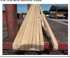
8. Once this wedge is in place the driver will then strap if possible the remaining bundle to the centre bars leaving the separated truss to be off loaded.
