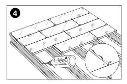
Repeat the application steps on subsequent rows of boards which should be laid in a staggered pattern. Short end joints, including perimeter edges, must fall on a secured joist or noggin. The boards must be fixed at the rate of three per board (i.e., one at each end and one in the middle). This nailing pattern gives a mechanical fixing every 1200 mm along each joist. Any excess adhesive should be left to dry then removed. If in doubt consult NHBC guidelines.
