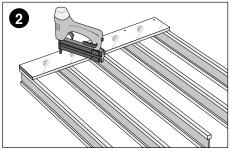
Mechanically fix the first row of boards over the joist using a fixing not less than 2  $\frac{1}{2}$  times the thickness of the board. Apply Kronobuild® D4 Adhesive along the open edge profile and joists in readiness for the next board to be fitted.
