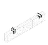
Gable restraint brackets placed on wall at 1200mm\* maximum centres (no fixings required).
