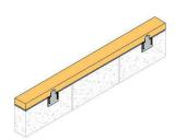
38-75mm wallplate bedded on mortar and fixed to gable restraint brackets with 3.5x40mm wood screws (2 no. per bracket).
