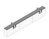
10mm maximum mortar bed on wall prior to wallplate being fixed.
